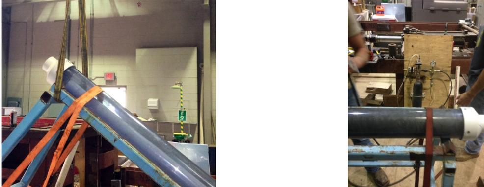
**Figure 7:** Lifting of the Setup Prior to Pouring of Drilling Fluid (left) and Set up with Drilling Fluid (right)
