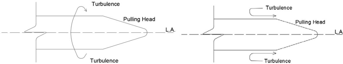
**Figure 11:** Turbulence on circumferential plane (left) and longitudinal plane (right)
