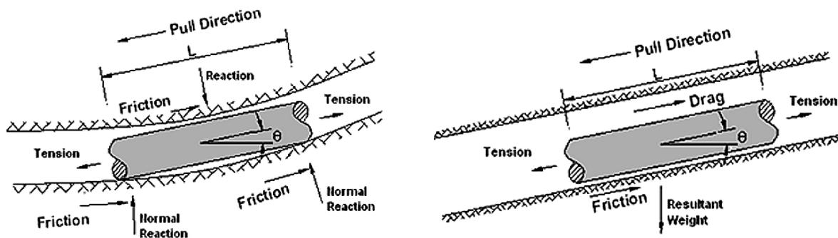
**Figure 1:** Pipe-Borehole Interaction during Pull Back in HDD Installation (after Huey et al., 1996) – Curved Section (Left) and Straight Section (Right).
