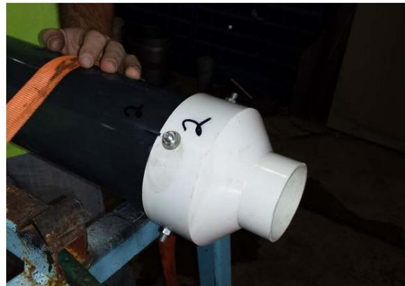
**Figure 4:** Drilling Holes on the Adapter and Pipe-A (left) and Adapter Attached to the Pipe-A (right)
