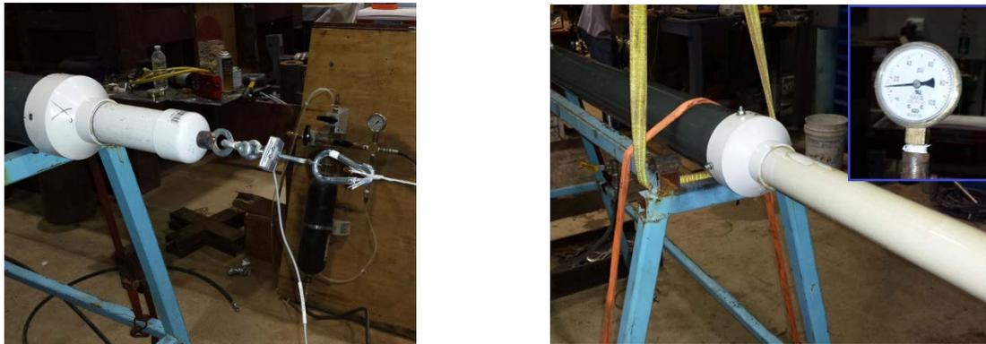
**Figure 8:** Pulling the Pipe-B (left) and Pipe-B pulled with applied of pressure (right)
