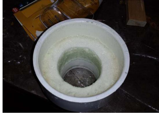
**Figure 3:** Removal of Inner Ring in a Lathe (left) and Trimmed Foam Layer inside the Adapter (right)
