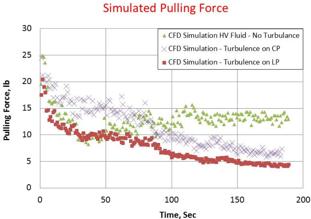
**Figure 12:** Reduction in pulling force due to turbulence
