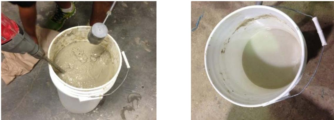
**Figure 6:** Preparation of Drilling Fluid (left) and Prepared Drilling Fluid (right)
