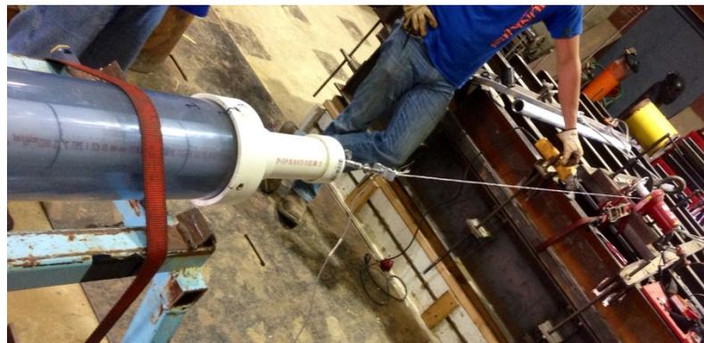
**Figure 5:** Setup Levelled (left) and Pipe-B Attached to a Winch Cable via the Load Cell (right)
