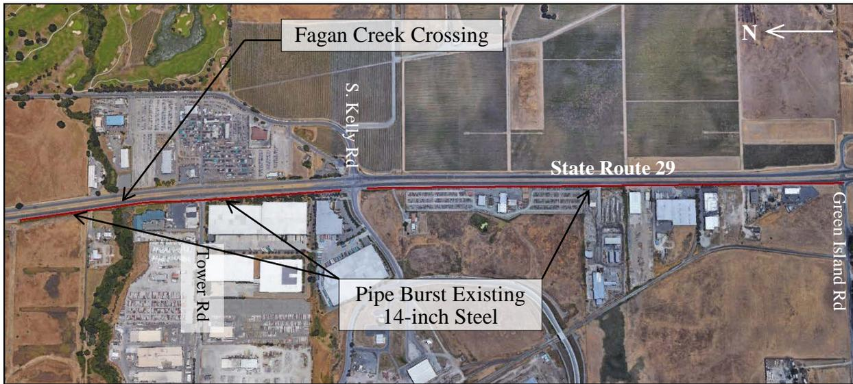
Figure 6. Extent of steel pipe alignment to be rehabilitated.
