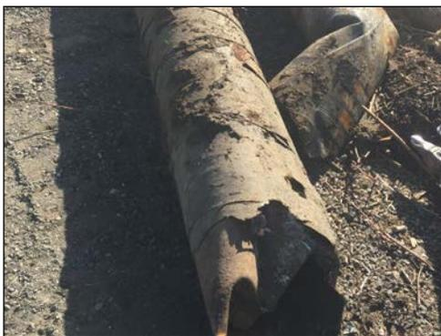
Figure 3. Existing 14-inch steel transmission main installed in the 1940s.
