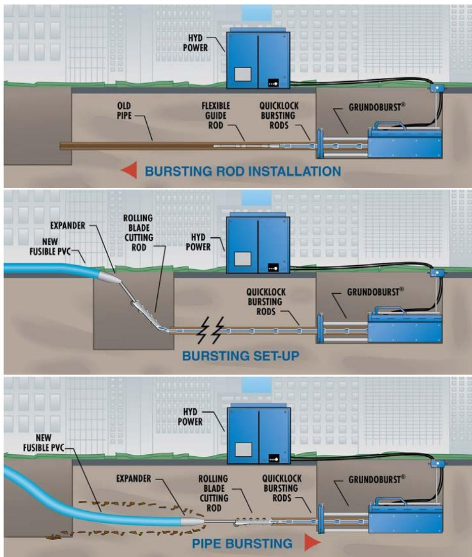
Figure 5. Step-by-step diagram of typical static pipe burst installation.
