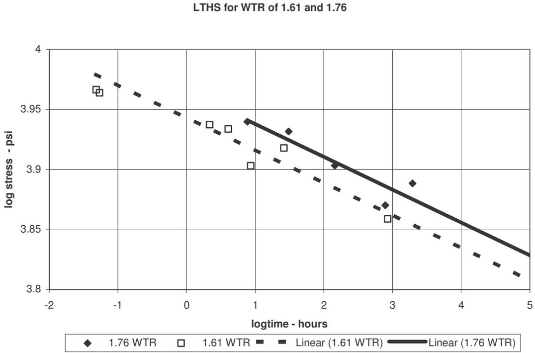
Repeating this testing using specimen sets with different wall thickness ratios allows us to plot HDB as a function of wall thickness ratio for a specific PVC formulation and expansion process. Figure 3 gives a projection based on the data currently available.
