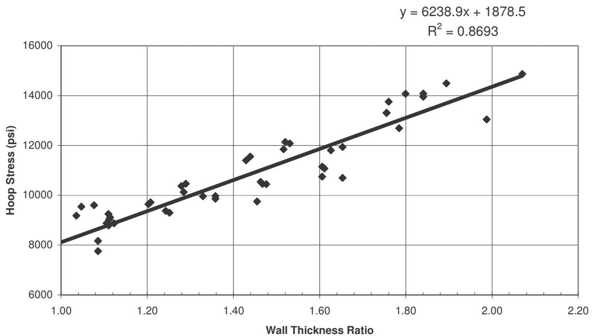
These results show that the short-term hoop tensile strength is strongly correlated with wall thickness ratio. Knowing the slope of the strength vs. wall thickness ratio line gives us the information we need to confirm that hydrostatic bursting of a pipe section will, even in a non-uniformly expanded pipe, occur at the location coincident with the minimum wall thickness, as the following calculation illustrates. The relationship
